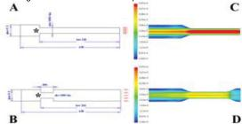
The simplified geometry of a percutaneous cannula (A), and a **smart**  $canula^{TM}$  (B) are compared by computational fluid dynamics (CFD). It can be shown, that higher velocities (red) occur in the long narrow segment (C) of a percutaneous cannula as compared to the zone of interest (\*) in the shorter constriction of a **smart**  $canula^{TM}$  (D) for an identical blood flow.
